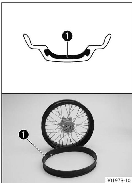
This vehicle uses a tubeless tire system in which a rim seal band ① is used instead of the conventional tube.
