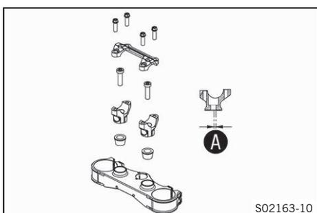
The holes on the handlebar support are placed at a distance of **A** from the center.
