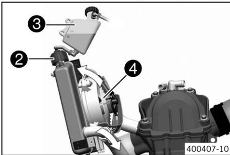
The coolant is cooled by the air stream and radiator fan ④, which is activated depending on the temperature.
