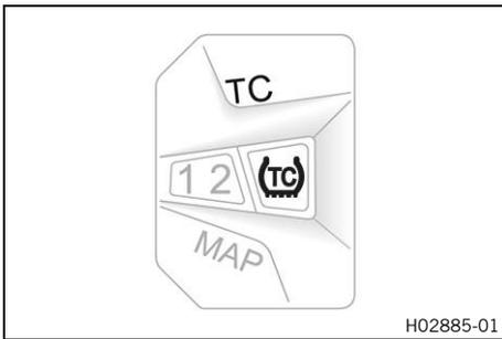
The motorcycle traction control (cornering MTC) lowers the engine torque in case of loss of traction in the rear wheel. Depending on the riding mode, different amounts of slip are allowed when the traction control is activated.
