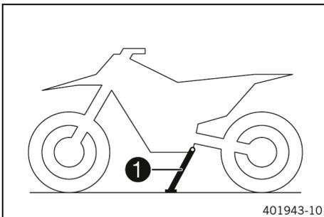
Side stand ① is located on the left of the vehicle. The side stand is used for parking the motorcycle.
