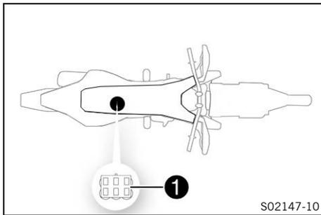
Diagnostics connector **1** is located under the engine electronics control unit.
