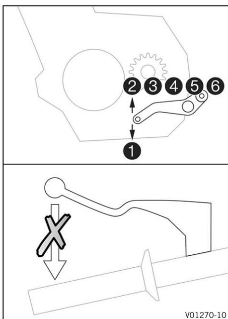
If the quickshifter + is activated, you can shift up and down without actuating the clutch. Because there is no need to close the throttle grip, uninterrupted gear shifts are possible. The quickshifter + uses the shifter shaft position to check whether or not a shift should be initiated, and sends a corresponding signal to the engine control.
