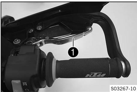
The hand brake lever **1** is fitted on the right side of the handlebar. The hand brake lever operates the front brake.
