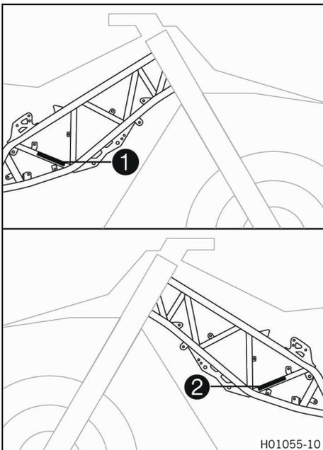
The Europe type label **1** is located on the right side of the frame. The Australia type label **2** is located on the left side of the frame.
