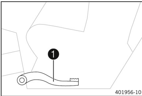
Foot brake lever ① is located in front of the right footrest. The rear brake is engaged with the foot brake lever.
